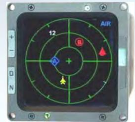
Astronautics' RWR display is also operating in full compatibility mode, allowing a Form, Fit & Function (FFF) **replacement to legacy systems that currently use CRT based display**. The significantly high-reliability (over 6,000 hours) display provides a significant Life Cycle Cost (LCC) improvement, compared to existing and difficult to maintain CRT based displays. The expected improvement is in a factor 30-40 times (!)
